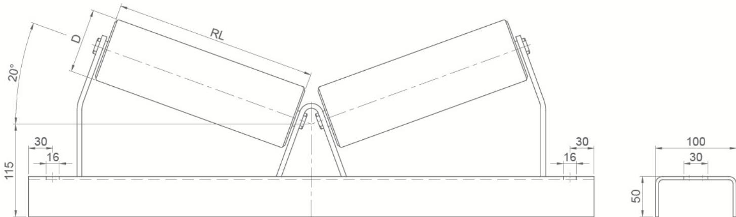
**Tube** :  $\varnothing$  63.5 mm,  $\varnothing$  80 mm,  $\varnothing$  89 mm,  $\varnothing$  108 mm
